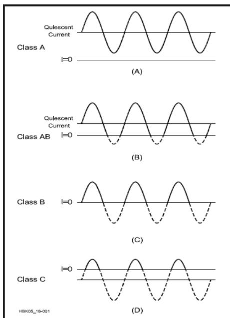
The class of operation of an amplifier stage is defined by its conduction angle, that is the portion of the sine wave drive cycle, in degrees, during which plate current (or collector or drain current in the case of transistors) flows. This, in turn, determines the amplifier's efficiency and linearity.
