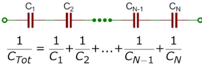
$$\frac{1}{C_{\text{Tot}}} = \frac{1}{C_1} + \frac{1}{C_2} + \dots + \frac{1}{C_{N-1}} + \frac{1}{C_N}$$
