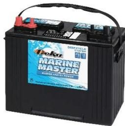
**Sealed Lead Acid batteries** – Gel Cells and AGM (Absorbed Glass Mat) batteries that are available in 12-volt versions (other Voltages are available but for Amateur Radio the 12-volt version is the most commonly used). They are sealed and use a “gelled” electrolyte and they can be operated in any position. They have current ratings ranging from smaller ones with a 1 ampere hour rating up to 80 ampere hours and more. These batteries are rechargeable.
