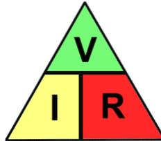
For example: if you have a 12-volt battery connected across a 6-ohm resistor the current flowing would be 2 amperes.
