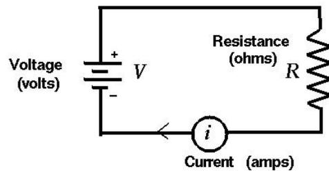
If we know the voltage and the resistance in a circuit, we can calculate the current that would be flowing using the following expression:
