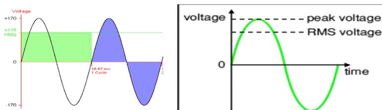
For a pure AC sine wave the equivalent RMS value is 0.707 times the peak value.
