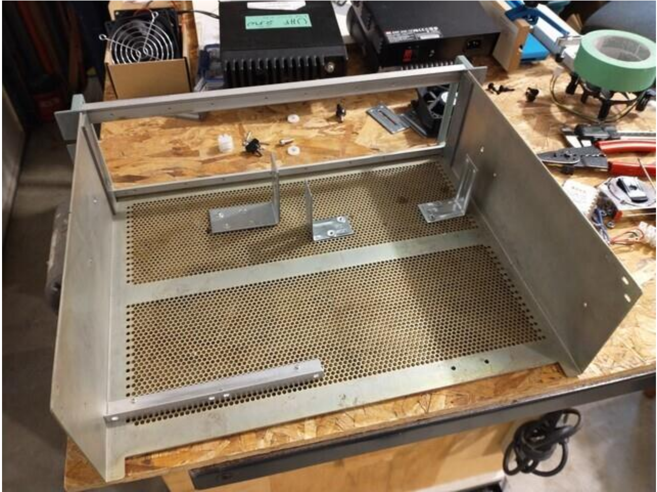
Rivet the brackets. Yes the two on the right are truss brackets from the lumber yard.
