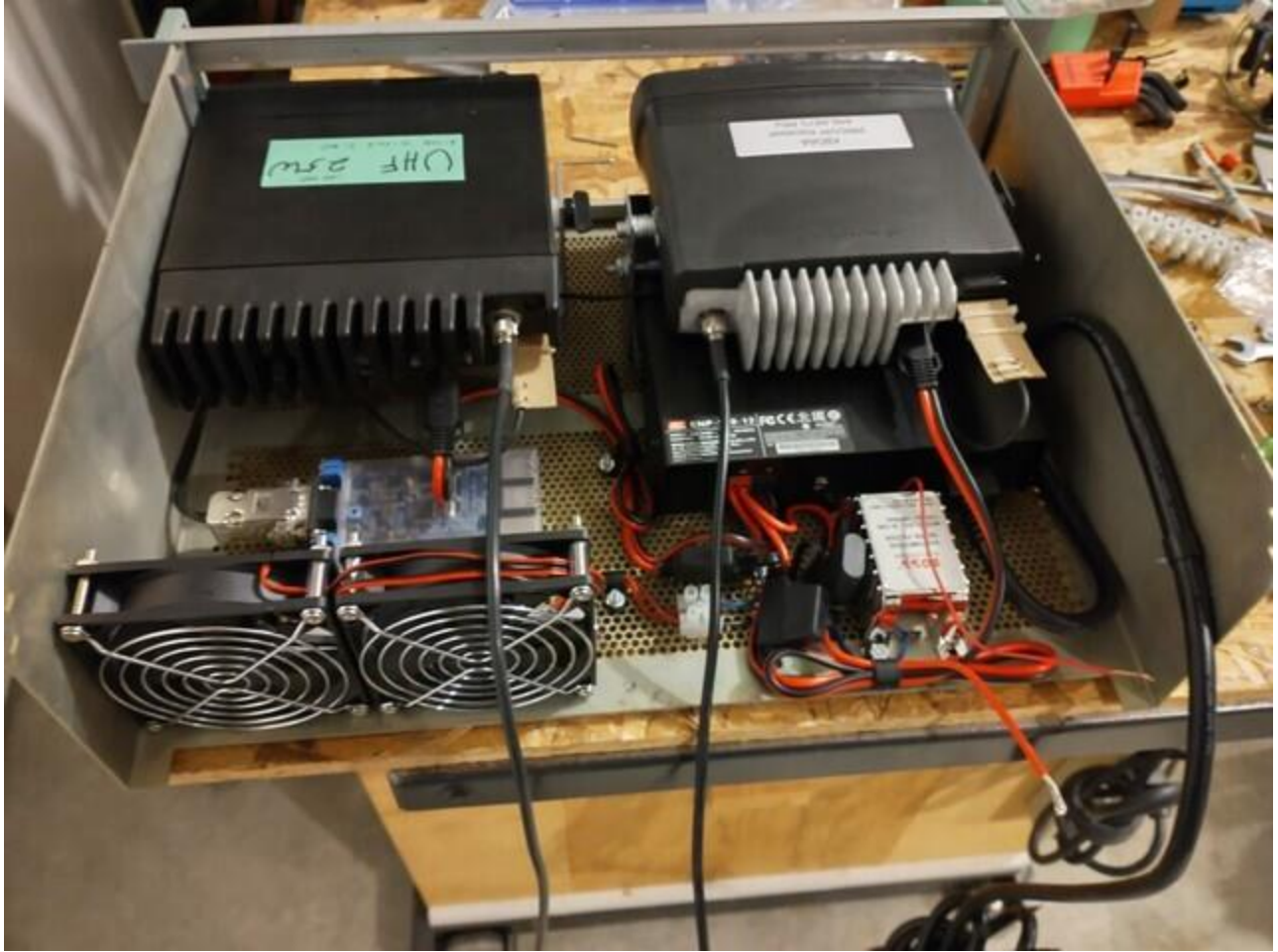
Add the RPi, fans, fan power filter, power cables, control cables and RF cables.
