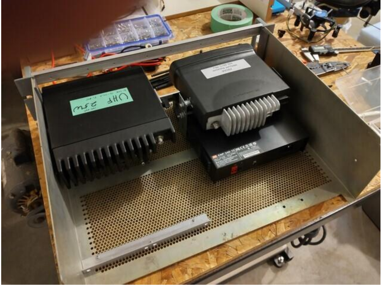
Radios and power supply mounted.
