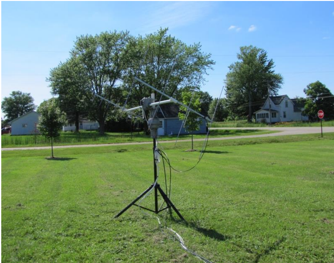
Azimuth-Elevation rotors and antennas for satellite work
