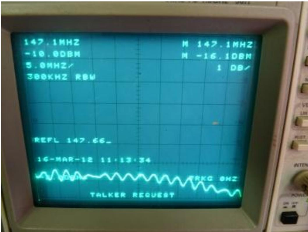
This is a picture of the feedline unterminated. It shows a reading of -16.1 DBm, which is the feed line loss, times two, from -13.6. This comes to 2.5 divided by 2, or 1.25 Db for the line, which is very good.
