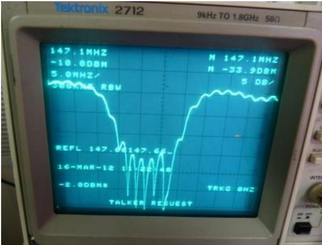
This is the new antenna, showing a return loss of 20.3 DB, (33.9 minus 13.6 reference).
