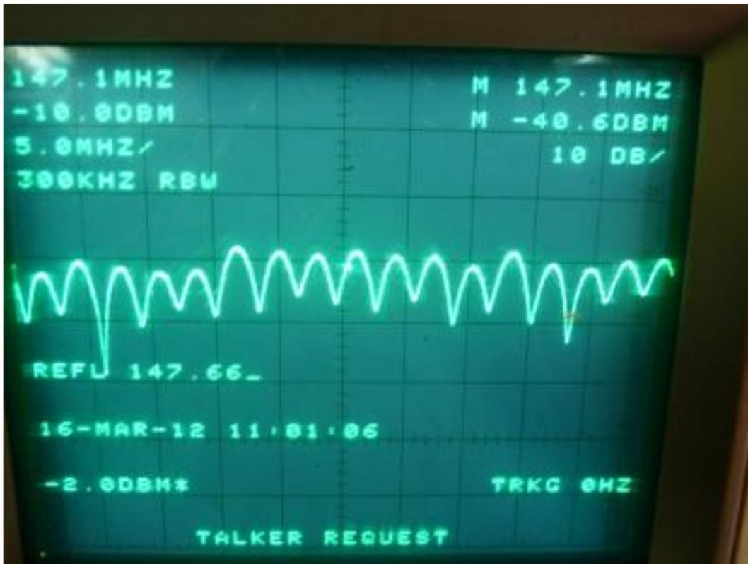
This is a picture of the feed line terminated with a 50 ohm load. A measurement of -40.6, a return loss of 27 db, or a VSWR of 1.09:1
