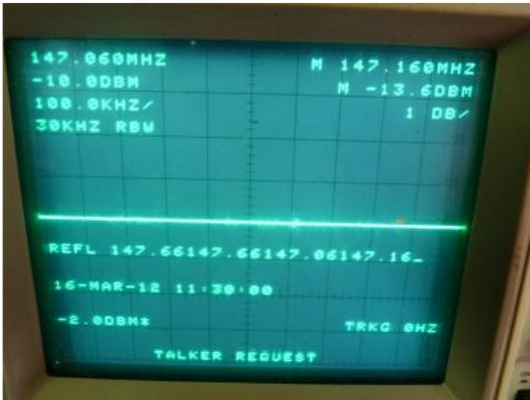
Explanation. This is a spectrum analyzer hooked up to a return loss bridge. This is a picture of the bridge with no load, a reference of -13.6 DBm on 2 meters.
